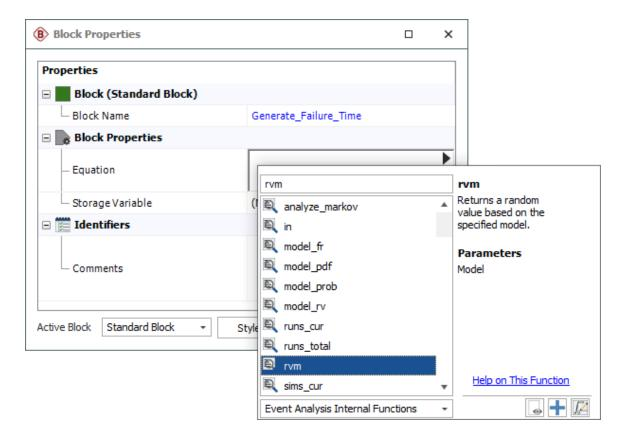
In the Enter Parameters window that appears, right-click in the **Model** field and open the Function Selector. Double-click the **Item\_Failure\_Distribution** model.
