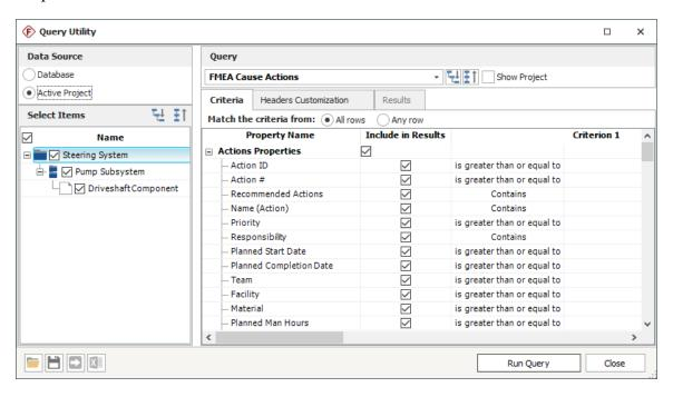
• You can then specify which columns you want to appear in the query results. For this example, clear the check box at the top of the Include in Results column, then select the individual check boxes for the following properties:
