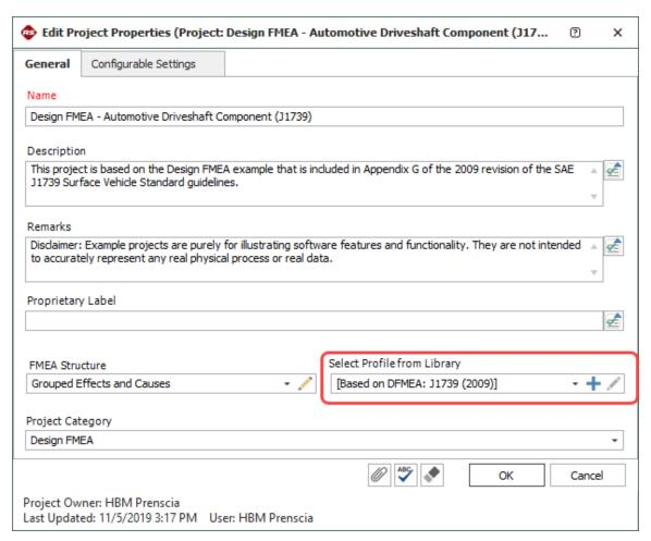
As you can see in the **Select Profile from Library** field, the configurable settings in this project are based on the DFMEA: J1739 (2009) profile. This predefined profile is shipped with the software and can be used to quickly configure the project to use the data fields and RPN rating scales specified in the 2009 revision of the SAE J1739 guidelines for Design FMEA (DFMEA).
